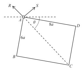
*ABCD* is a uniform rectangular lamina with mass *m* and sides AB = 6a and AD = 8a. The lamina rotates freely in a vertical plane about a fixed horizontal axis passing through *A*, and it is released from rest in the position with *D* vertically above *A*. When the diagonal *AC* makes an angle  $\theta$  below the horizontal, the force acting on the lamina at *A* has components *R* parallel to *CA* and *S* perpendicular to *CA* (see diagram).
