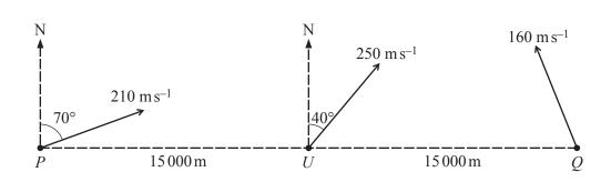
An unidentified aircraft U is flying horizontally with constant velocity  $250 \text{ m s}^{-1}$  in the direction with bearing 040°. Two spotter planes P and Q are flying horizontally at the same height as U, and at one instant P is 15000 m due west of U, and Q is 15000 m due east of U (see diagram).
